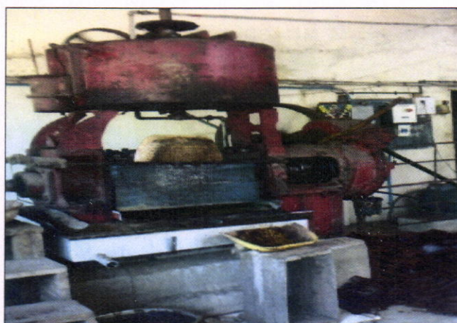
Oil Expeller (Screw press type) used by cottage industry 10
