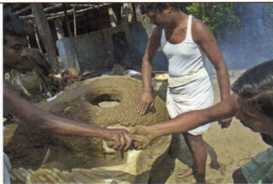
Workers sealing and covering a wax mould of an icon with clay.
