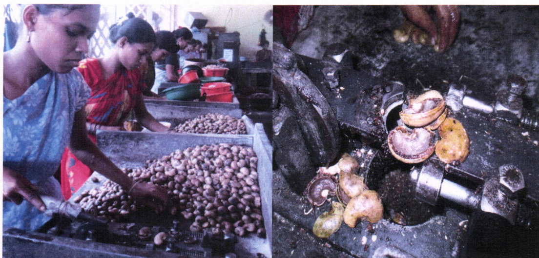
Cashew nuts cutting with help of machines.
