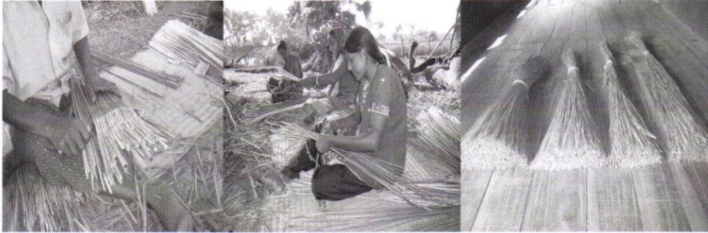
Figure: Processing of harvested Madur kathi ; i) Cutting of Madur kathi into strip by using special knife ii) Bundling of splitted strips by women iii) Different grades of bundeled strips.
